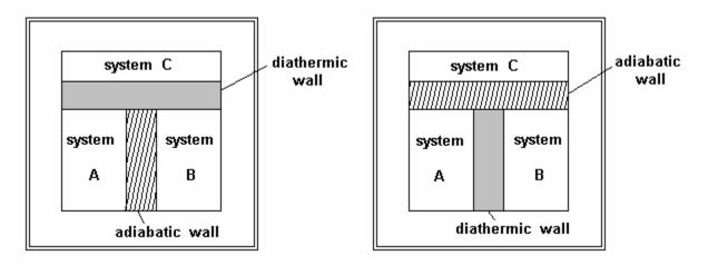
Suppose, as shown in the first figure, systems A and B are separated by an adiabatic wall and both are in contact with system C through a diathermic wall. An insulating wall covers the whole device. It is experimentally observed that after systems A and B have attained thermal equilibrium with C, if the adiabatic wall between the systems A and B is replaced by a diathermic wall, no changes occur in systems A and B indicating that they are in thermal equilibrium with each other.
