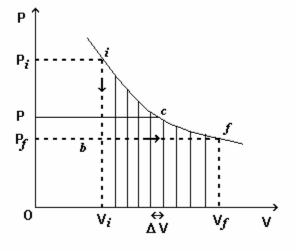
The work done by the gas is the area enclosed by  $P \rightarrow V$  curve as shown in the figure. Work is an extensive variable as it is the product of one extensive variable (V) and other intensive variable (P).
