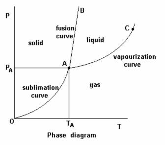
gas phases co-exist in equilibrium. Similarly, AC is a vapourization curve, points on which indicate the pressures and temperatures, at which liquid and gas phases co-exist in equilibrium.
