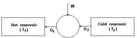
Schematic representation of a heat pump/refrigerator
