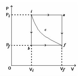
of heat, spends energy W to do work and the balance Q - W increases its internal energy.
